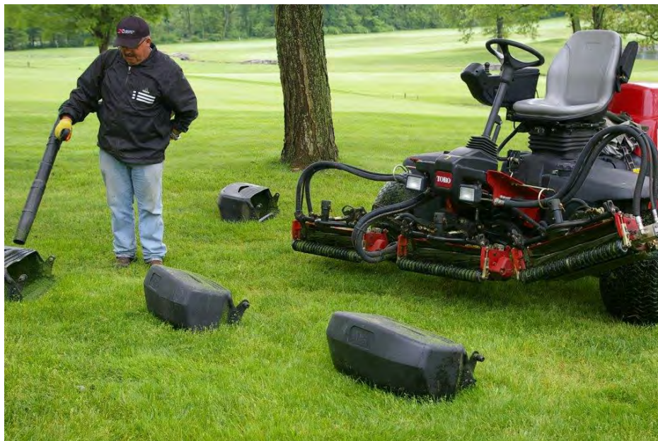
Figure 31. Blowing clippings off equipment prior to washing.
