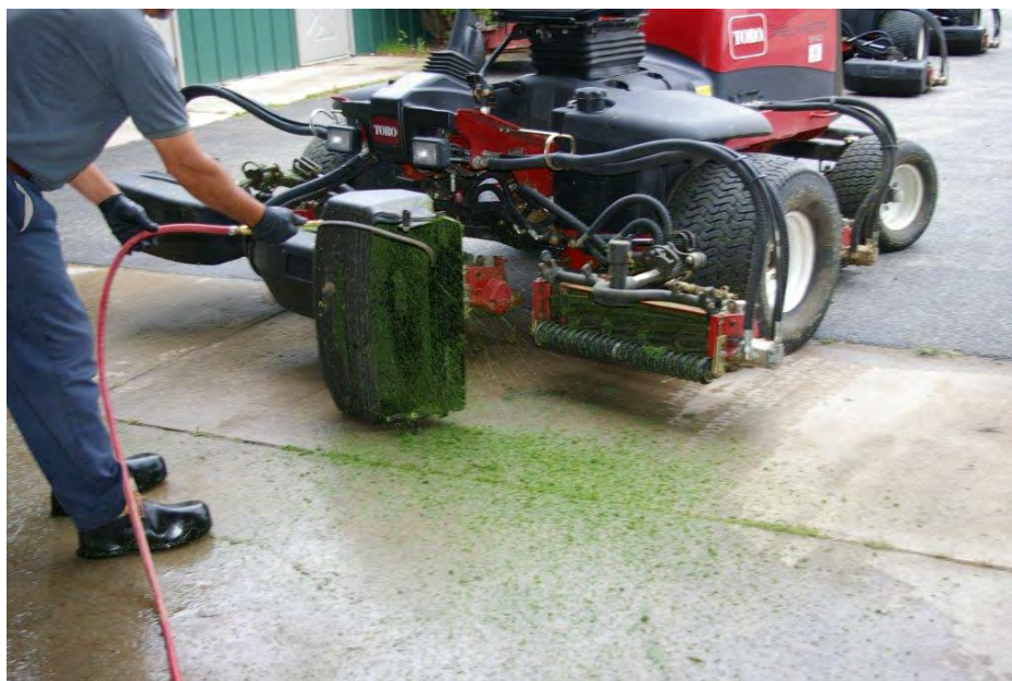
Figure 32. Equipment prewash on clippings collection pad.
