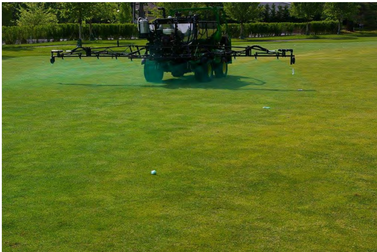
Figure 23. Fairway pesticide application using foam and dye for accuracy.
