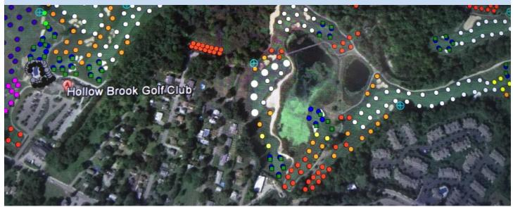
Interactive map of every sprinkler head on the golf course. The user can select a sprinkler head to run or can visualize which ones will run. The highlighted white dots are heads that are within an instant program created just for high sides of fairways, which need more water than the flat surfaces.
