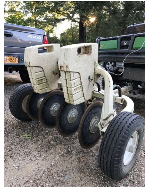
Figure 1. Veris 1000 sensor used to map soils at the case study site.
